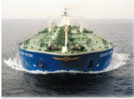
During 1998, six vlccs were brought into ABS class including the 300,155 dwt GOLDEN VICTORY built to SafeHull criteria by Hitachi Zosen for Golden Ocean.
