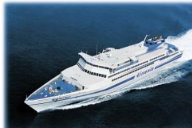
The world's fastest monohull ferries, built at Fincantieri to ABS class for Tirrenia, entered service in 1998. These 11,400 gross ton passenger and vehicle ferries have a service speed of 41 knots.
