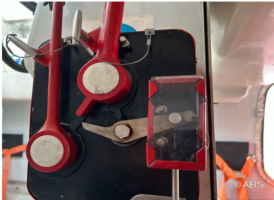
Lifeboat hydrostatic release not engaged and reset
