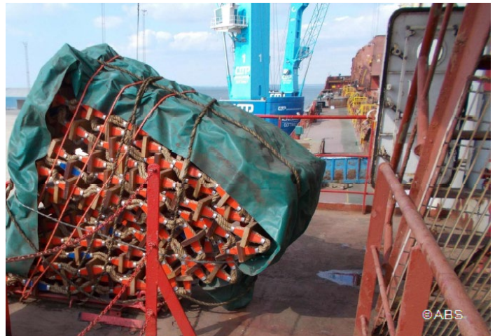
Improper stowage of embarkation ladder
