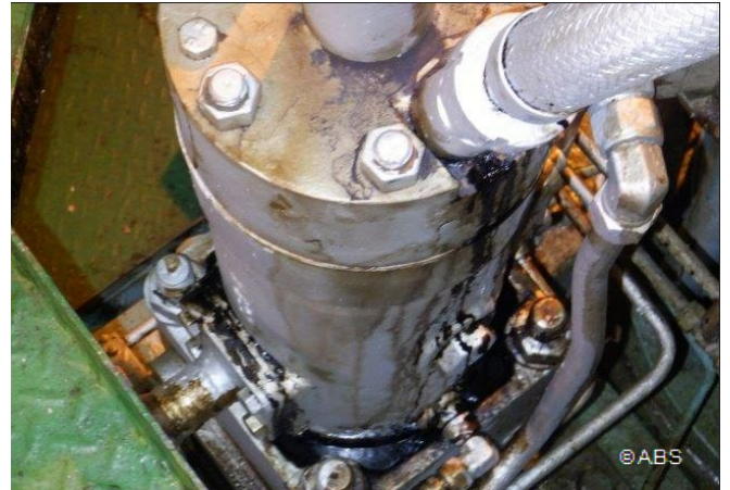
Main Engine Fuel Pump Leaking
