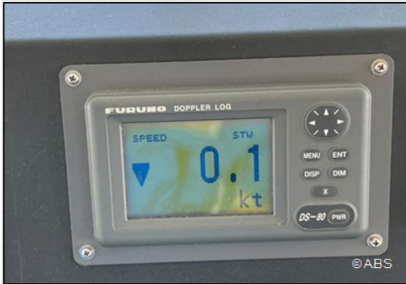
Speed and distance device is inoperative
