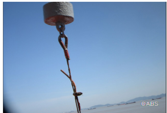
Lifeboat remote launching mechanism is not working while operating from inside of the boat
