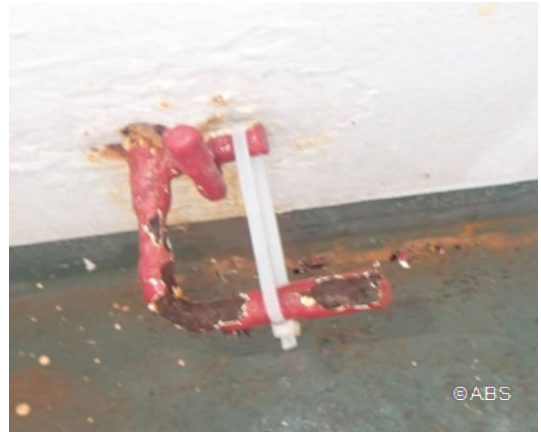
Man Overboard Buoy (MOB) unable to release due to operating mechanism stuck caused by wasted handle
